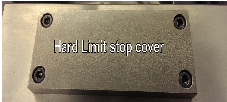
Illustration 1: Hard stop cover. Remove only if table can't be rotated off the hard stop.
